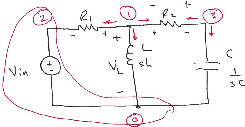
$$V_2 = V_{in} \quad \text{source constraint}$$
