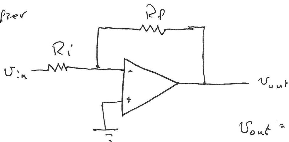
$$v_{out} = -\frac{R_f}{R_i} v_{in}$$
